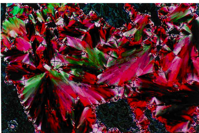
Figure 1. Textures of a 4.8 mol % mixture of ( \pm )- 2-d 6 in PhB observed by polarized microscopy (100 \times ): homeotropic and fan textures of the SmA phase at 70°C (top); Schlieren and broken fan textures of the SmC phase at 68°C (bottom).
