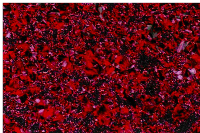
Figure 2. Textures of a 9.1 mol % mixture of ( \pm )- 2-d 6 in PhB observed by polarized microscopy (100 \times ): broken fan/Schlieren texture of the SmC phase with coexisting isotropic domains at 67°C (top); uniform broken fan/Schlieren texture of the SmC phase at 61°C (bottom).
